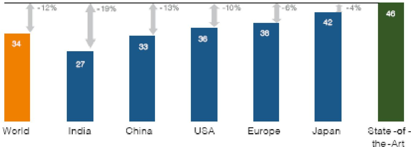
NOTE: The total installed capacity of steam power plants in Europe is around 2,300 GW (2011) and 40% will be retired in the next two decades, indicating 1,000 GW capacity needs to be replaced. With an average global coal fired plant efficiency of 34%, it becomes obvious that there is a huge efficiency potential.
